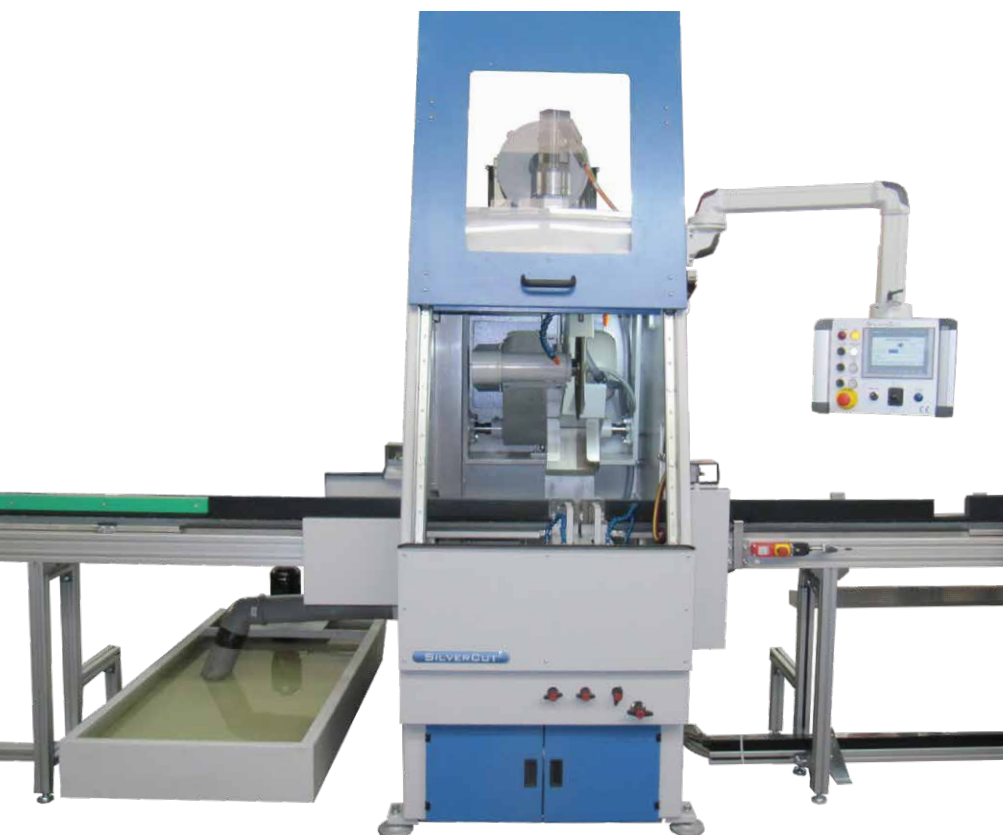
Control panel with touch Display and joysticks for all servo axes of the cutting wheel.
