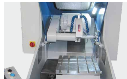
Big inside space with long axes movement. Alu-table for good corrosion resistance.
